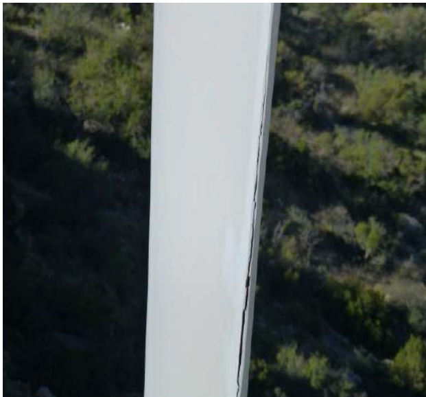
Figure A. Longitudinal cracks found on the trailing edge of a wind turbine blade.
