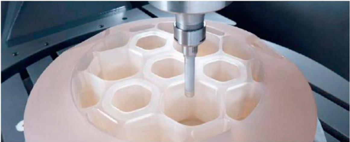
Fig. 1 Mirror support with thin-walled light-weight structures made from Zerodur ® using ultrasonic machining
