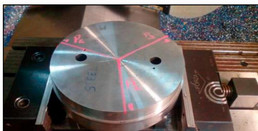
Fig1. (a) Details of roughness measurement points on the steel block; (b) Roughness measurement set-up.
