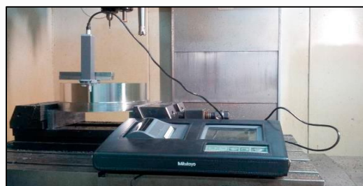
Fig1. (a) Details of roughness measurement points on the steel block; (b) Roughness measurement set-up.
