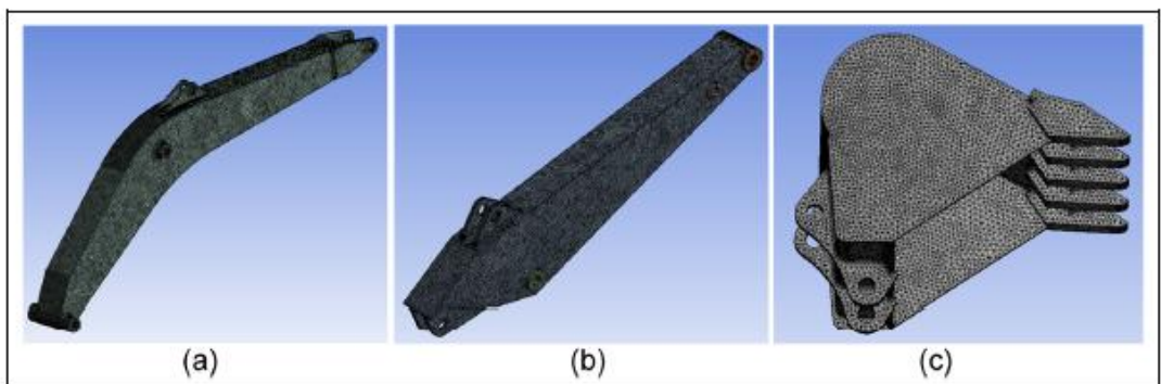
Figure 2. Finite element model of the working device: (a) boom model; (b) arm model; and (c) bucket model.
